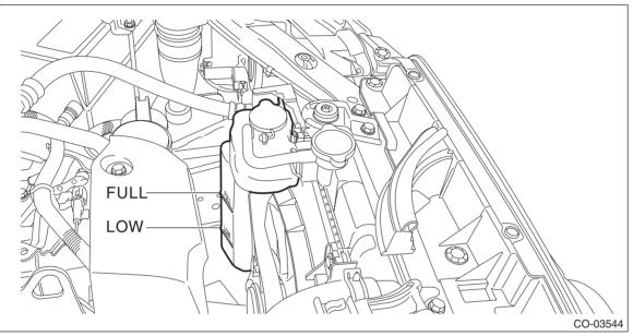
4) Close the radiator cap and start the engine. Race 5 to 6 times at 3,000 r/min or less, then stop the engine. (Complete this operation within 40 seconds.)
